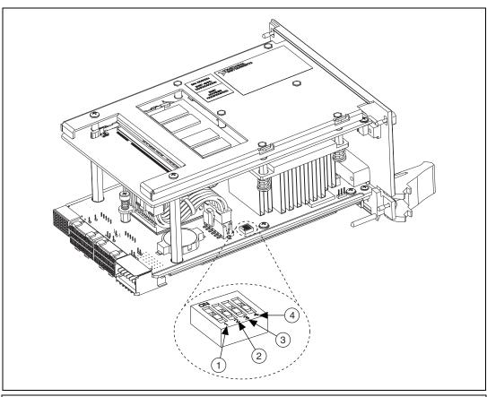
1 Switch 1—Boot LabVIEW RT 2 Switch 2—Boot Safe Mode
